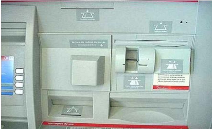
The equipment as it appears installed over the normal ATM bank slot.
